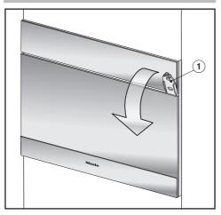
■ Insert the opener included with the appliance ① about 3 cm into the gap between the door and the control panel on the right-hand side and then pull the door open.
