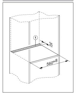
■ Create a cut-out ① in the intermediate shelf where the combination steam oven is to be placed.
