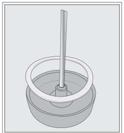
If necessary, you can remove the connecting piece and sealing ring from the milk container lid. Once you have removed the stainless steel tube, the connecting piece is easy to push out from the inside of the lid.
