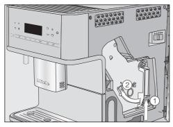
Press and hold the button on the end of the brew unit handle ① and, whilst doing so, turn the handle to the left ②.
