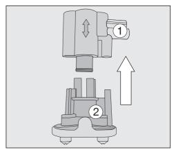
■ Pull the upper silicone section with the aperture for the milk pipework ① off the black holder ②.
