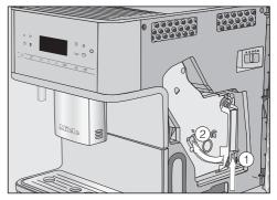
Press and hold the button on the end of the brew unit handle ① and, whilst doing so, turn the handle to the left ②.
